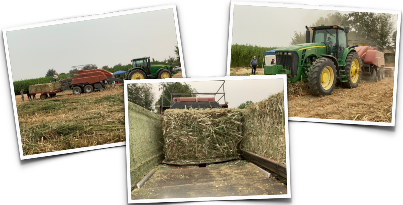
Hemp was easily baled using traditional straw baling equipment
