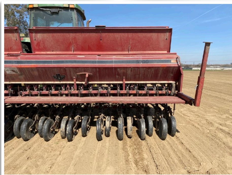
This grain drill spaced the crops 7" apart in neat rows
