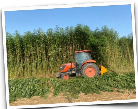
The sickle mower worked best at cutting the stalks
